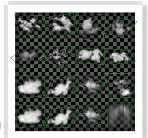
We come up with a particle trimming algorithm for reducing the amount of fillrate waste when rendering particles. This method ended up improving our cloud and particle rendering performance by more than 2x. For details, refer to the "Graphics Gems for Games: Findings From Avalanche Studios" talk in the "Advances in Real-Time Rendering In Games" course.
